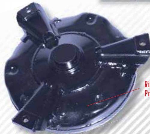
Tack Welded High Stress Areas
