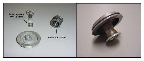
When reassembling transmission with servo's in their proper place you must make these adjustments. Set bands at  $2\,\%$  turns for rear band &  $2\,1/8$  turns for the front band. A 3.8 Intermediate Band Lever is preferred lever to use for this set-up. The clutch pack for the High/Rev. must have .070"-.080" clearance. The forward clutch pack must have .030"-.040" clearance in it.
