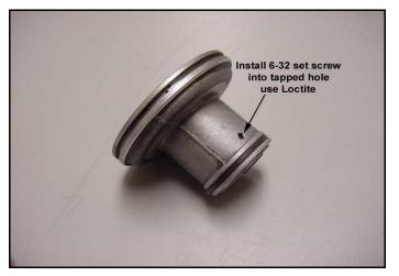
When servo is disassembled, use the #36 drill bit to drill bleed hole out. Then use the 6-32NC tap to tap the hole. CAUTION DO NOT TAP ALL THE WAY THROUGH THE HOLE. Because set screw will bottom out on pin & will mess with the pin placement.
