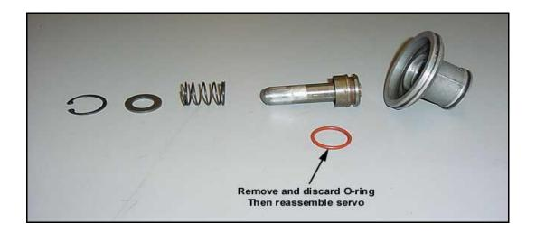
Before reassembling 2<sup>nd</sup> band servo. Remove and discard O-ring on pin, it will no longer be needed. After O-ring is removed reassemble servo back together.
