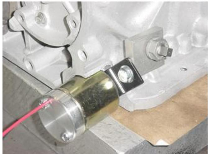
8. Install the new Trans-Brake valve body in the case, make sure manual valve is properly positioned with shift lever. Proper bolt torque is crucial to the operation of this valve body. Torque the valve body to case bolts at 100 in-lbs., Torque the long filter bolts at 70 in-lbs.
